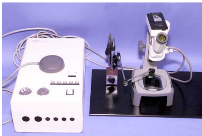
Figure 1. Diagram and photograph of fundus photography equipment. Upper panel: Basic features of fundus photography equipment. Lower panel: Photograph of actual equipment. The large white box on the left is the power supply. The foot pedal, which is normally placed on the floor, is resting on top of the power supply.
